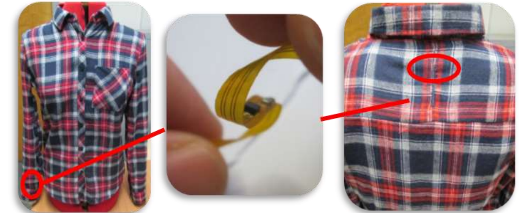
Motion sensing garments (UoS) (Li et al - Sensors 2020, 20(18), 503310)
