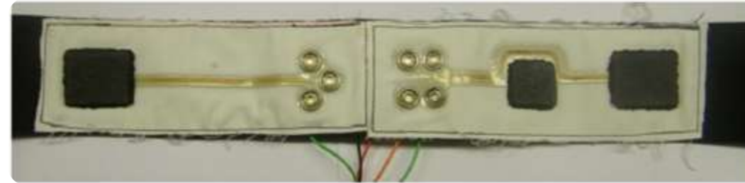
Printed Active electrodes on fabric (UoS) (Paul et al 2015 Sens. & Act. A. 221, p60-66410)
