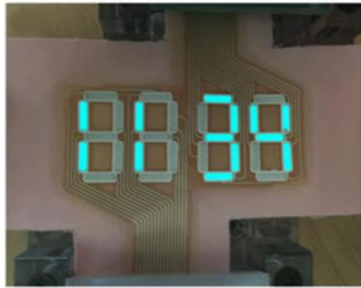
Printed Electroluminescent Watch Display on Fabric (UoS) (M. de Vos et al (2016) J. of Display Tech. 12: 757-1763.)
