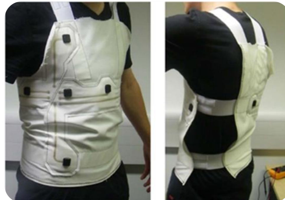
Printed frank configuration vest (UoS) (Paul et al 2017 Smart Mater. Struct. 26 025029)
