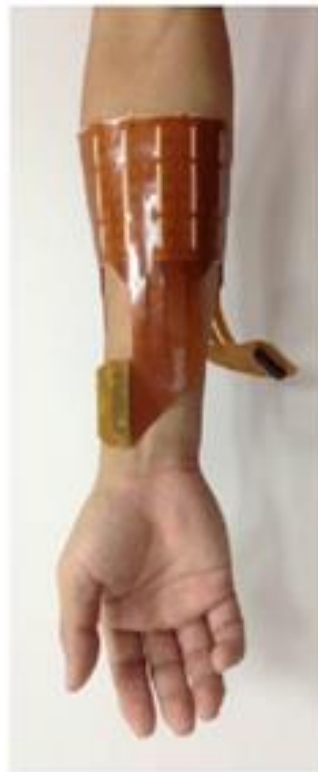
Etched copper EMG electrode array on plastic
