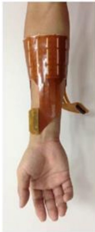
Etched copper EMG electrode array on plastic
