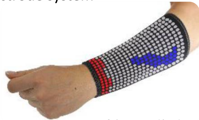
WEARPLEX concept of 'virtual' electrodes
