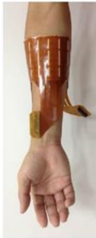
Etched copper EMG electrode array on plastic
